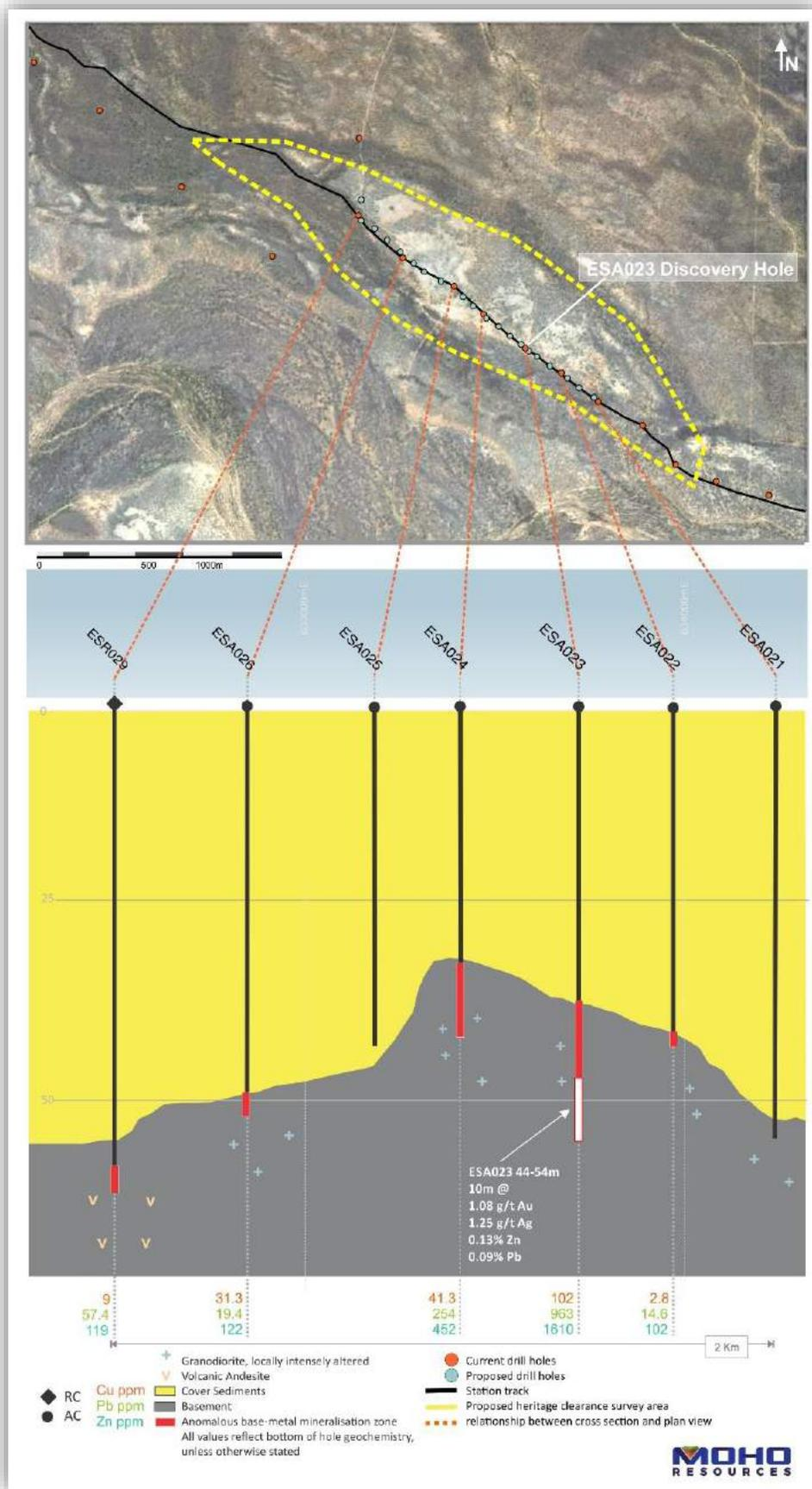
Figure 3: Cross Section of the Arrowhead Prospect showing Pronounced Basement High
