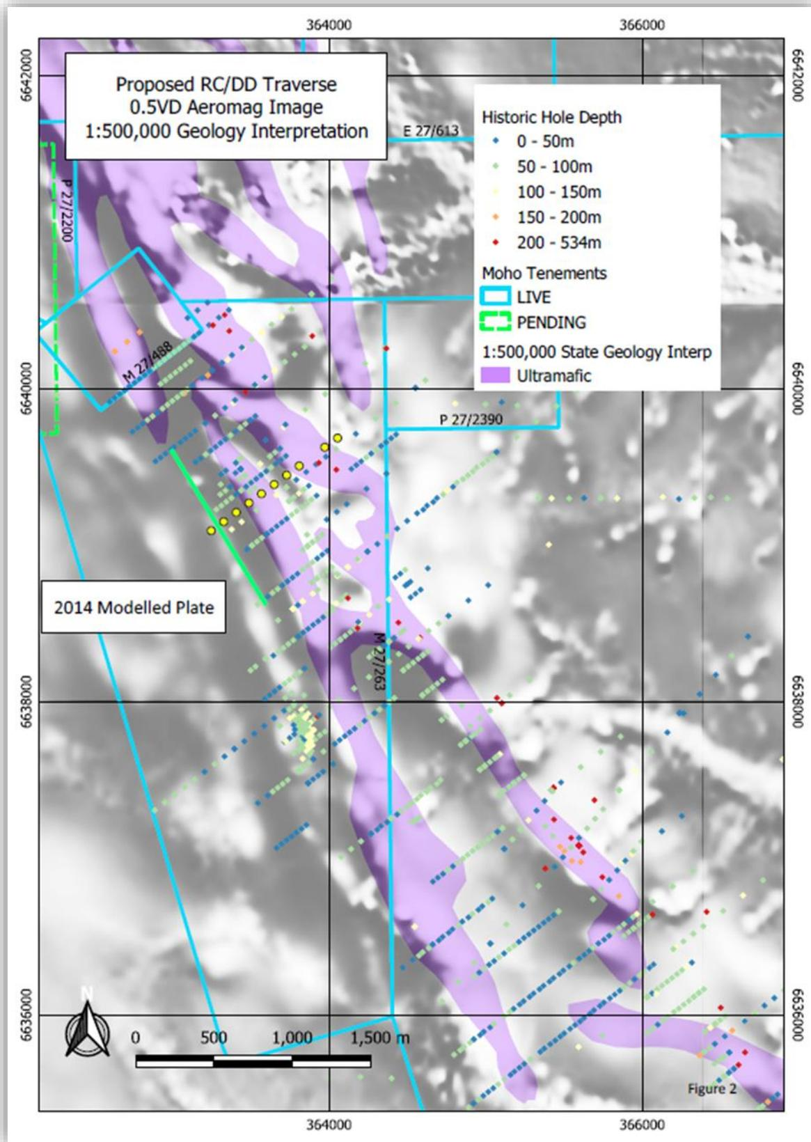
**Figure 2: Location of proposed RC and diamond drill hole traverse in relation to modelled EM conductor plate at Omrah target and historic drilling (overlain on ultramafic geology interpreted from magnetics)**
