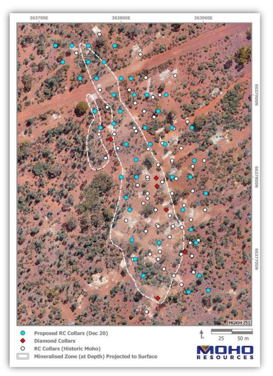
Figure 5: Proposed collar locations of Phase 2 RC drill program in relation to previous RC and diamond drilling and known mineralisation at East Sampson Dam
