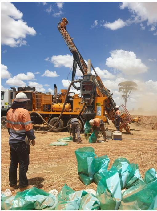
Figure 4: RC drilling, Burracoppin, January 2021
